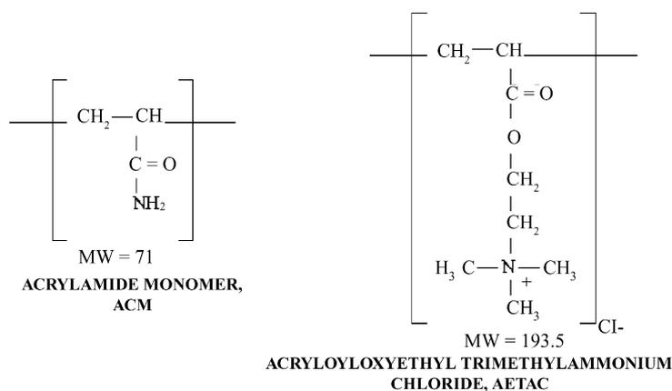
Fig. 1. The structure of polymer used Percol 757, 80% cationic copolymer (ACM/AETAC), molecular mass  $\sim 1.8 \times 10^6$ .
