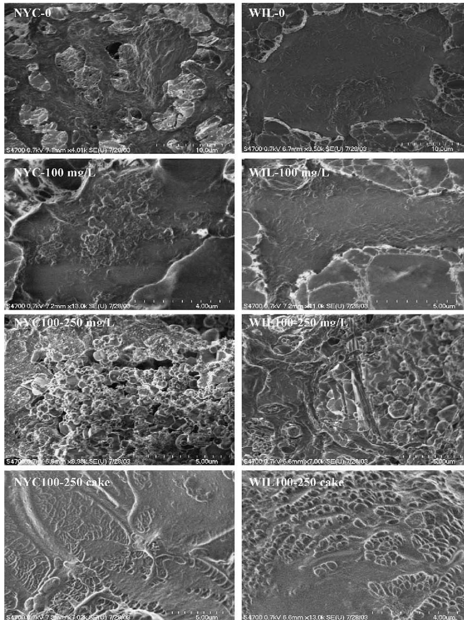
Fig. 12. SEM images for NYC (left) and WIL (right) biosolids samples: (a) raw, (b) enzyme treated (100 mg/L), (c) enzyme treated and polymer flocculated (250 mg/L), and (d) final cake product.
